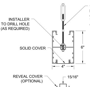
1/4-20 LH/RH THREADED ROD & TURNBUCKLE ASSEMBLY (ALL HARDWARE ABOVE TURNBUCKLE BY OTHERS)
